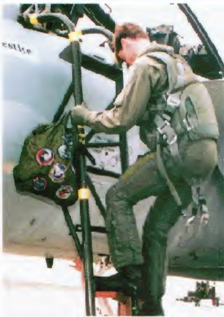
The USAF Advanced Technology Anti-G Suit (ATAGS), is a full coverage uniform pressure system designed to more effectively prevent pooling of blood in the lower body
